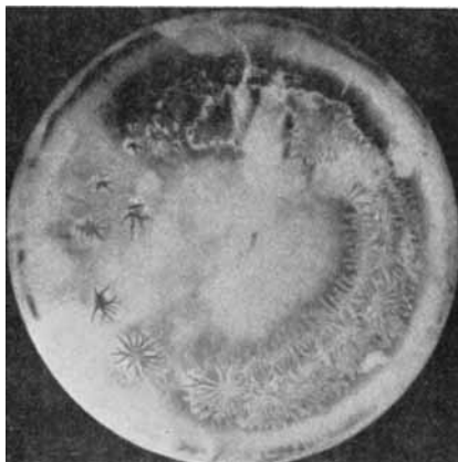
Fig. 1. Very high charge (unrubbed white polystyrene).
